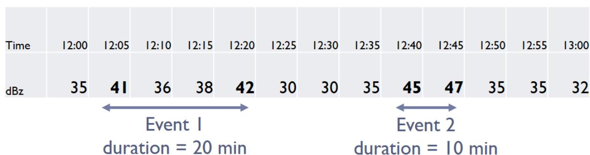
Fig. 6: Example of the storm event duration definition.
