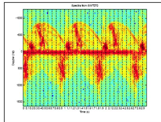
**Fig. 1.b:** Time variation (3s) of the Doppler spectrum of an Enercon E66 wind mill for a 39° rotor orientation (QuinetiQ, 2003).
