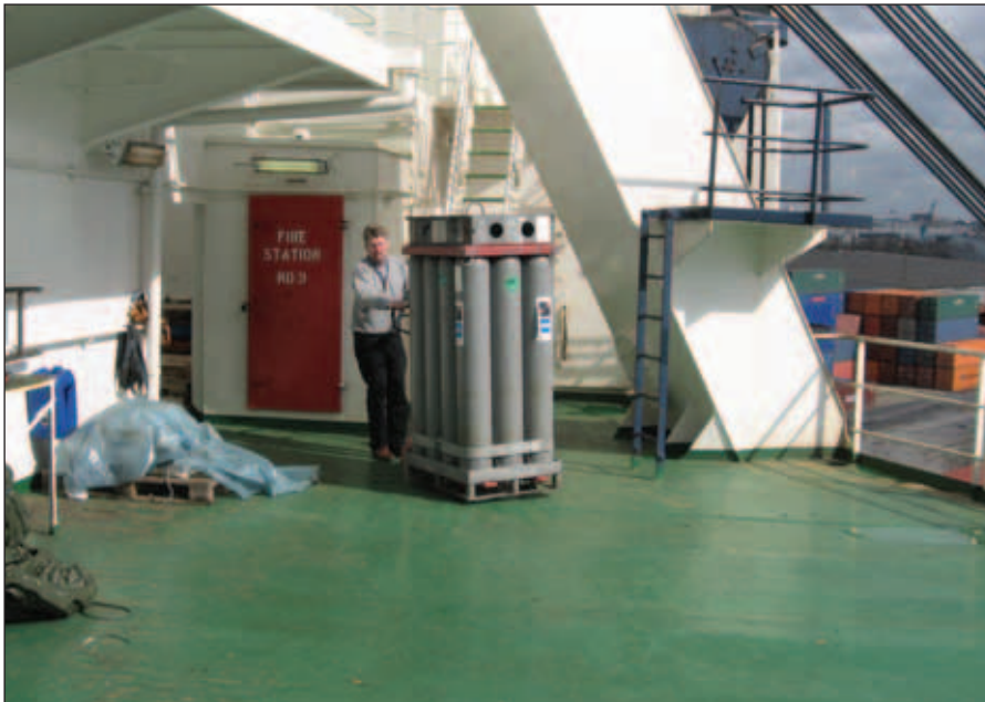
▲ Helium loading: preparing helium bank for weather balloon operations
